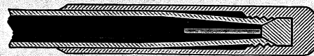
No. 8. Sectional view of cap, showing cone in the tip which plugs end of nozzle, making it air tight.
